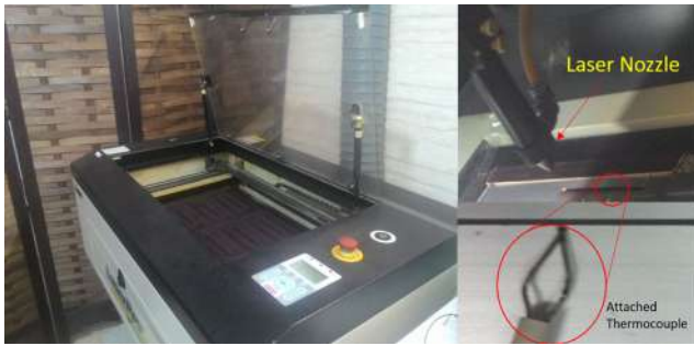
Fig. 5 Photo of the experimental setup of the laser cutting and thermocouples location
