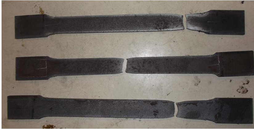
Figure 9. Three failed specimens under tensile loading
