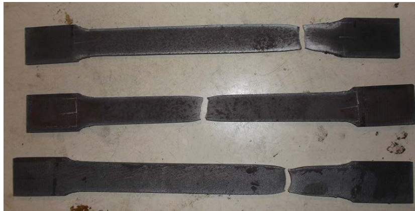
Figure 9. Three failed specimens under tensile loading
