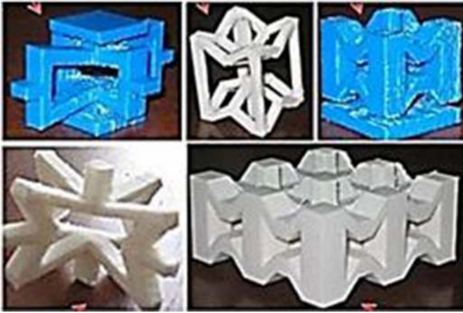
Fig. 2. Some of the structures fabricated by 3D printing machine.
